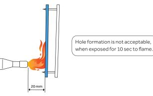
SaFR<sup>™</sup> fibre pass the surface ignition test as NO hole formed in the SaFR<sup>™</sup> fibre
