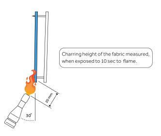
The **SaFR™** fibre had shorter char lengths (35–40 mm) compared to other cellulosic FR fabrics (120mm-160mm).
