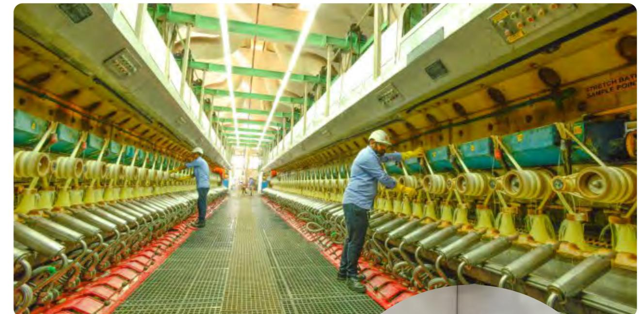
**Furthermore, the Lyocell fibre is produced using a unique solvent spinning method distinguished by its inherent closed-loop process and solvent recovery rate of more than 99.7%**
